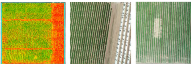
Fig. 2. A quicktile mosaic image of the surveyed field of green beans (left), drive way and plastic mulch with other crop (middle) on the right side of the mosaic image in red, and a plant missing spot (right) of a yellow rectangular shape close to the mid-bottom of the mosaic image.
