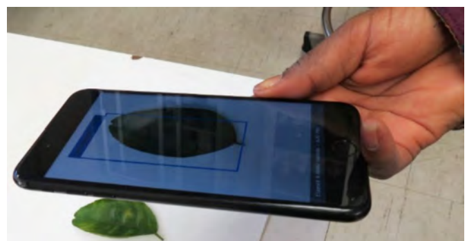
Fig. 2 (below). The prototype iPhone app being used to diagnose citrus greasy spot disease in less than one second.
