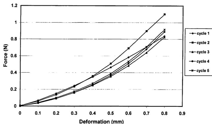
Figure 7. Force-deformation curves for fruit #4. Compression cycles 1 and 2 were performed 25 s apart. Subsequent cycles were performed at 15-min intervals.
